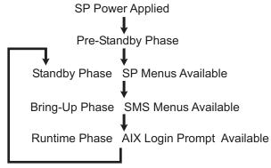
**Pre-Standby Phase:** This phase is entered when the server is connected to a power source. The server may or may not be fully powered on. This phase is exited when the Power-On Self-Tests (POSTs) and configurations tasks are completed.
